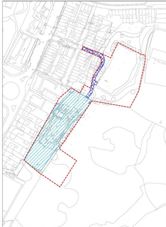
EXISTING IMPERMEABLE AREA APPROX SCALE 1:1000
